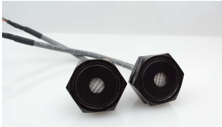
Figure 41 Photograph of Nexceris Lion Tamer AWARE prototype.
