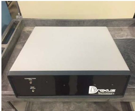
Figure 40 Photograph of Dynexus Technology inline Rapid Impedance Spectroscopy prototype.
