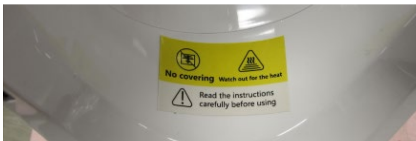
Figure 8. Non-compliant with UL 1278, section 67.14 warning label.
