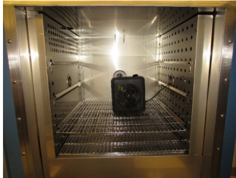
Figure 4.3. Heater inside the conditioning oven
