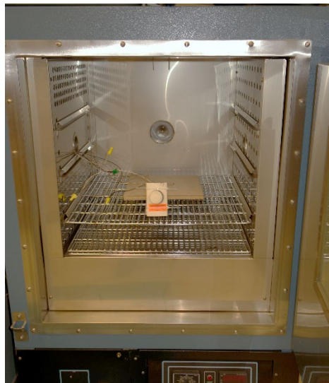
Figure 4.11. Thermostat in the conditioning oven
