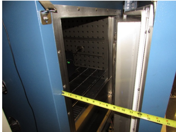
Figure 4.6. Oven chamber door partially opened about 9 inches (23 cm)
