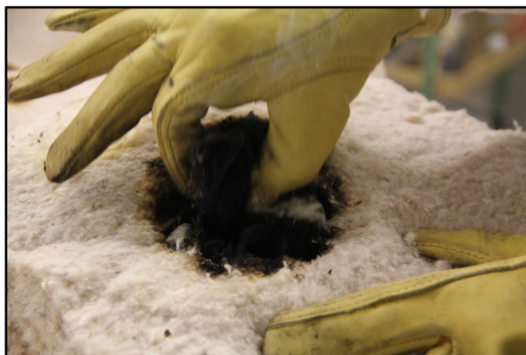
Figure 31. Removal of charred felt.
