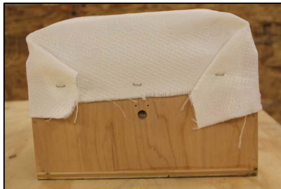
Figure 27. Ticking fastened, using staples.
