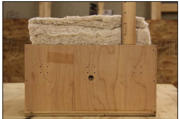
Figure 24. Cotton felt in test box, protruding up to 3 in. from the top of the box.
