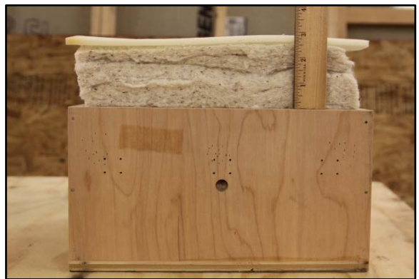
Figure 25. Urethane foam placed over cotton felt.
