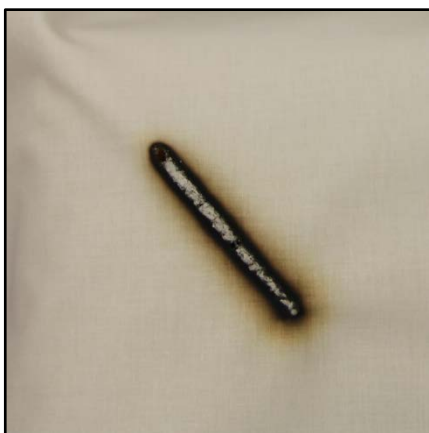
Figure 29. Pass result example on ticking.
