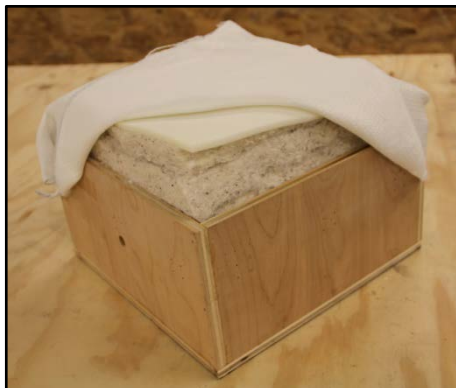
Figure 26. View of ticking, urethane foam and cotton felt partially fastened.
