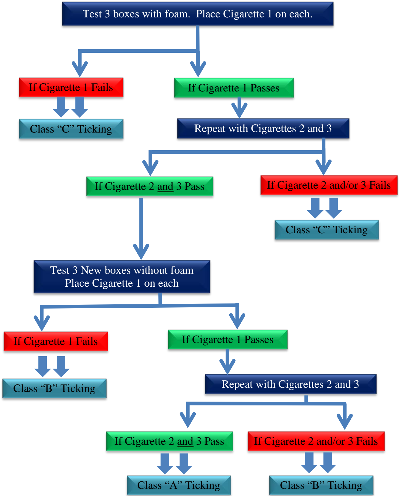
Figure 23. Flow diagram to determine Ticking Classification.
