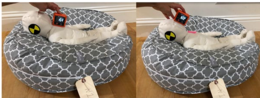
Figure 6. Photos of torso (left) and head (right) segment measurements of the newborn CAMI dummy in a normal Leachco Podster product.
